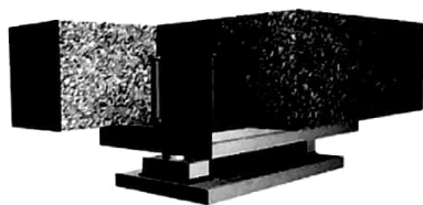
concrete superstructure (deck) - bearing no. 1.6 fixed in all directions (V) - anchoring plate with anchoring studs
